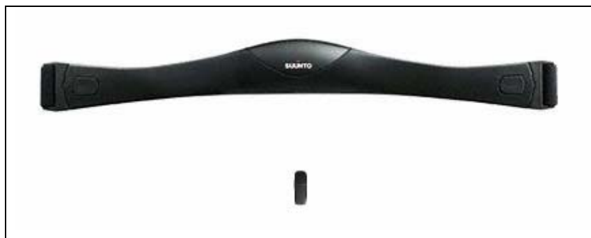
Fig. 1 - SUUNTO Heart rate monitor consisting of a thorax belt and a USB radio receiver
